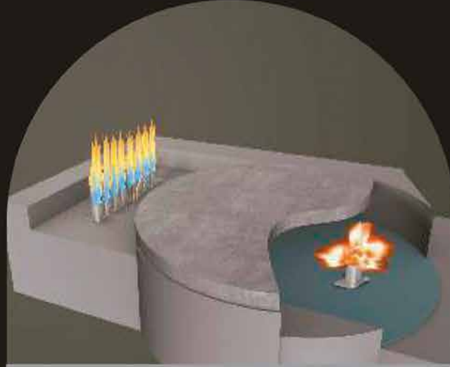
sub-plate cooking gas burner
